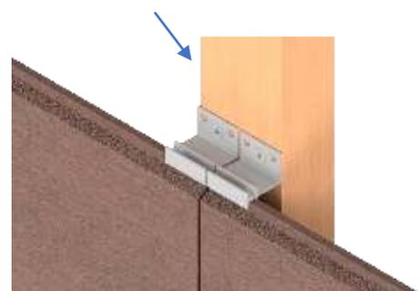
The façade profile may protrude a maximum of 50 mm beyond the end of the substructure at the end of the façade.
