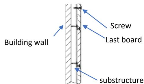
Substructure 60mm +
